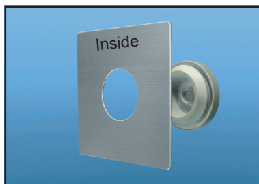
Push the grommet into the hole.
