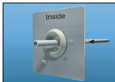
Pierce the grommet with the cable.
